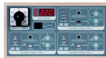
► Three phase equipment synoptic (Independent phase regulation)
